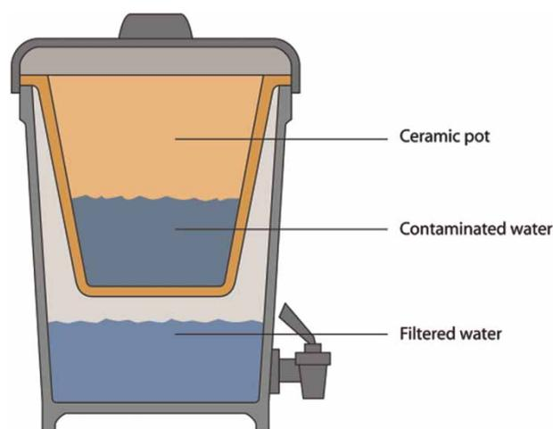
Figure 1 | Ceramic pot filter with receptacle.
