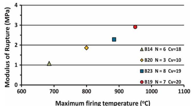
**Figure 8** | Average MoR versus maximum firing temperature.
