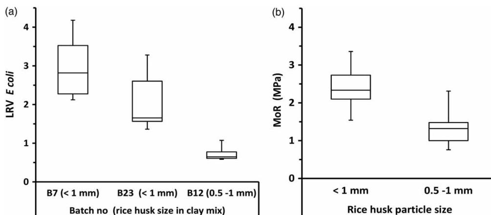
**Figure 9** | Box-and-whisker plots of LRV and MoR for pots with different rice husk particle sizes. (a) LRV for pots with different rice husk particles; (b) MoR for pots with different rice husk particles.
